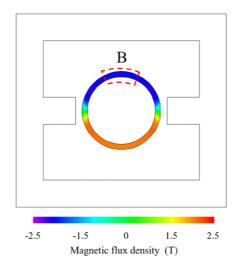
Fig. 6. Distribution of  $B_{\theta}$  in the section of the steel pipe.
