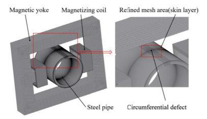
Fig. 3. 3D FEA model with refined mesh area.
