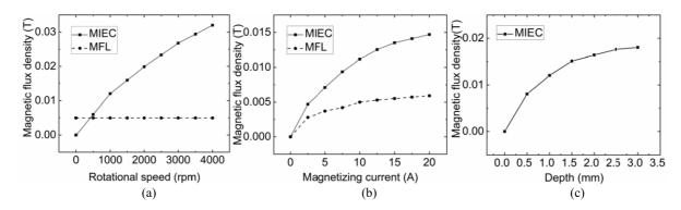
Fig. 7. MIEC perturbation magnetic field signal amplitude (a) and MFL signal amplitude at different rotational speeds; (b) and MFL signal amplitude at different magnetizing current; (c) at different depths.
