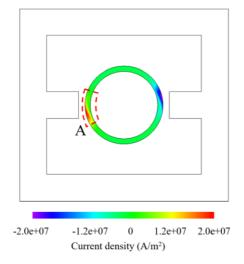
Fig. 5. MIEC distribution in the section of the steel pipe.
