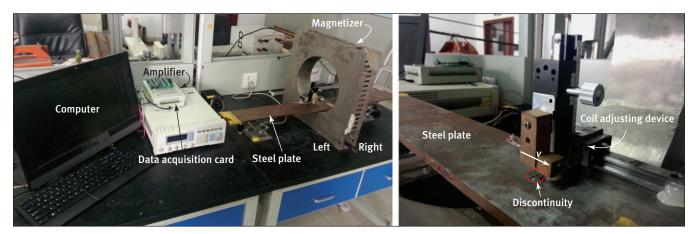
Figure 16. Two views of the MFL instruments for steel plate testing.
