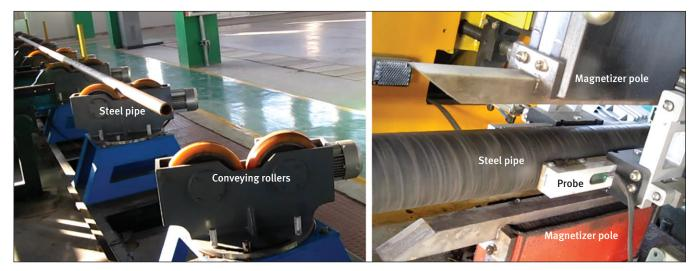
Figure 1. Two views of the MFL inspection apparatus for steel pipes.
